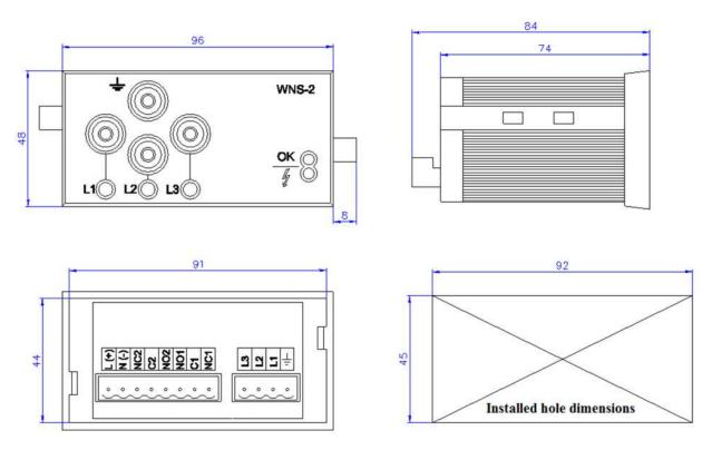
Fig.3. Dimensional drawings of voltage indicator.
