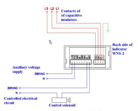
Fig. 2. Wiring of voltage indicator with blockage.
