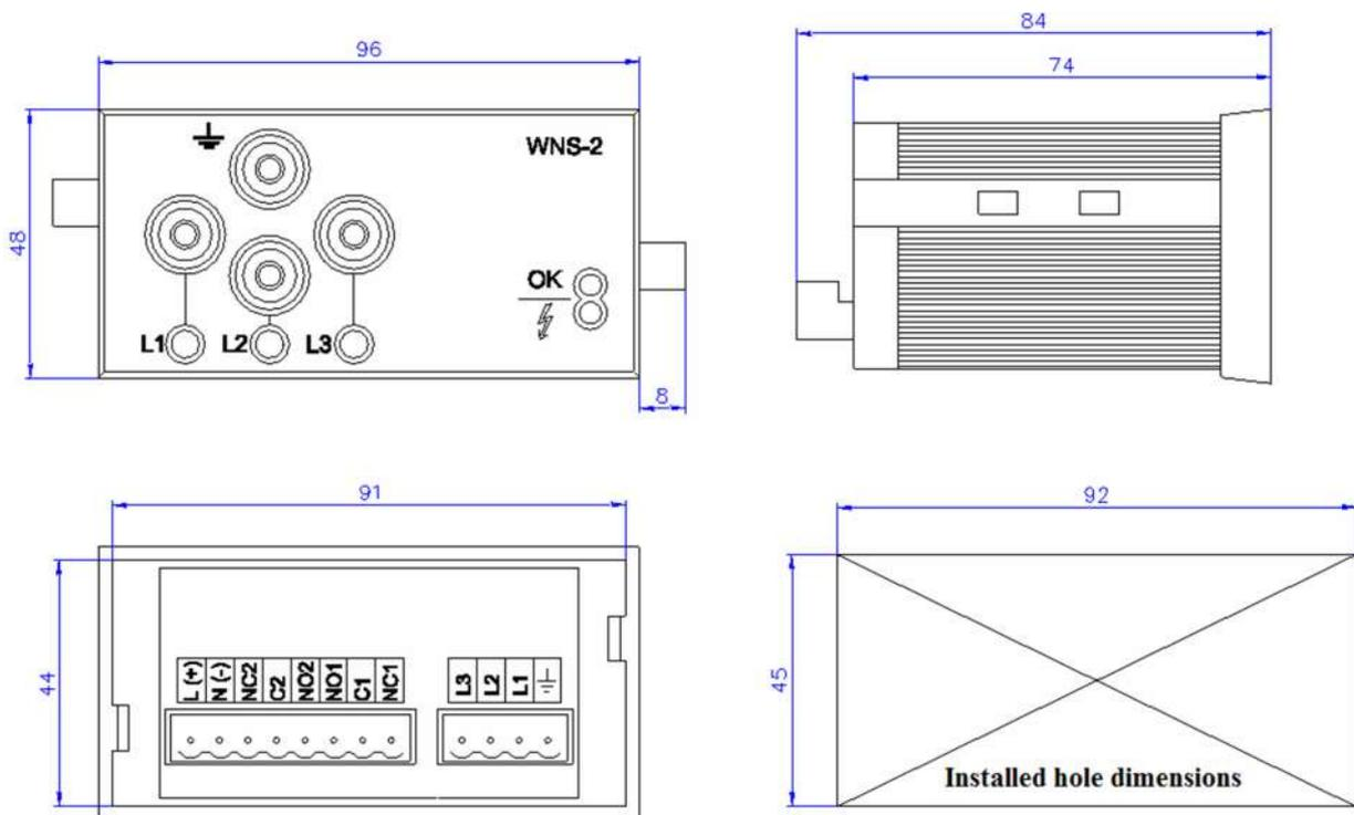
Fig.3. Dimensional drawings of voltage indicator.
