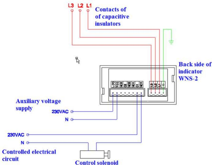
Fig. 2. Wiring of voltage indicator with blockage.
